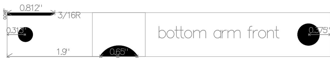
Radius cut with 3/4 EM both parts separated by 3/8"
